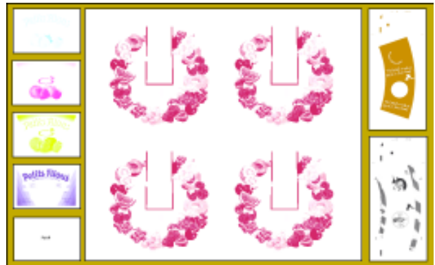
The Nexus RIP supports a whole range of flexo-specific functions such as layouting of color separations on a printing form.
